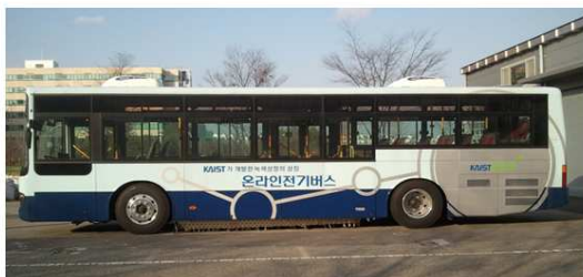
Fig. 1 The on-line electric vehicle
