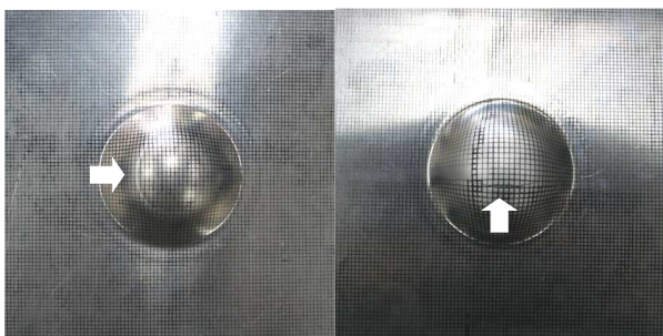
(d) 200mm (e) 200mm (with lubricant) Fig. 2 FLD specimen after experiment
