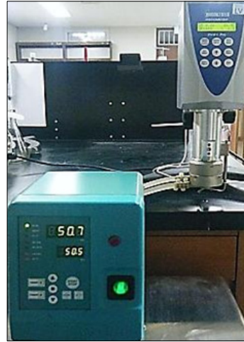
Figure 1: Experimental apparatus for viscosity measurement.
