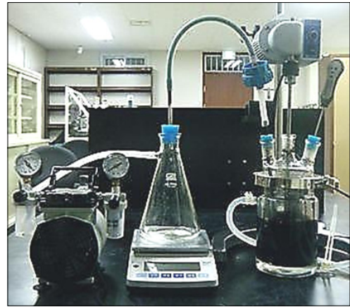
Figure 9: Experimental apparatus for WAT measurement by filter-plugging method.
