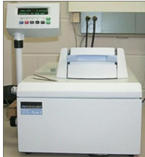
Figure 6: Differential scanning calorimetry for WAT measurement.
