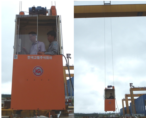
Figure 11: Prototype tower service lift system and performance test.
