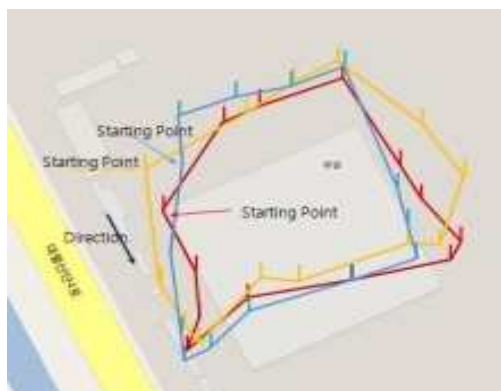
b) Using an external DGPS component
