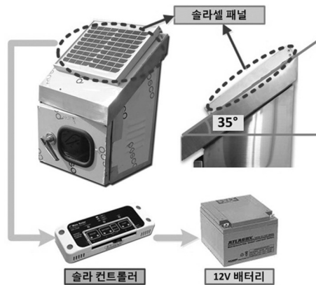
Fig. 4. Self-energy generation using solar cell panel.
