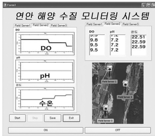
Fig. 11. Monitoring system for the water quality measurement in wireless sensor network.
