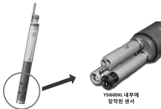
Fig. 3. Internal sensors of YSI600XL.
