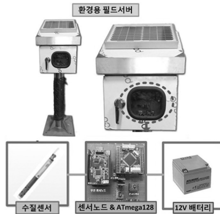
Fig. 2. The structure of field server for the portable water quality monitoring system.
