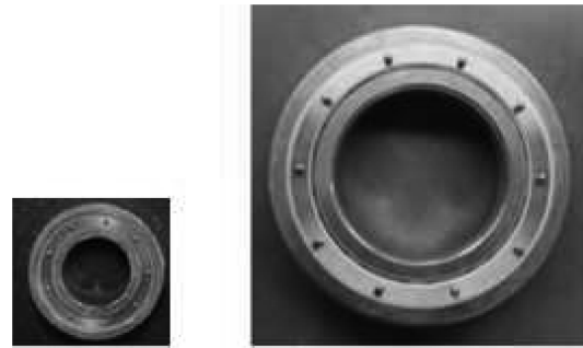
Fig. 3. Ball bearings used in the test (left: 6205, right: 6214).
