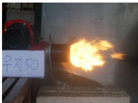
Figure 3. Scenes of flame size measurement and exhaust gas analysis.
