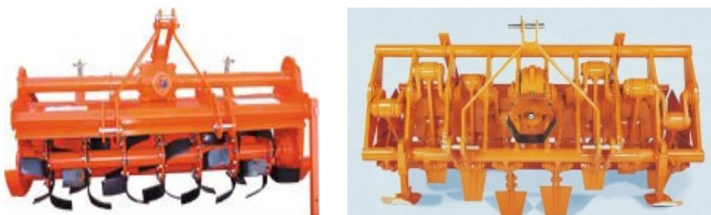
**Figure 1.** A view of rotary and crank type of rotavators.
