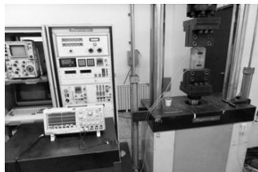
Fig. 6 Fatigue test machine
