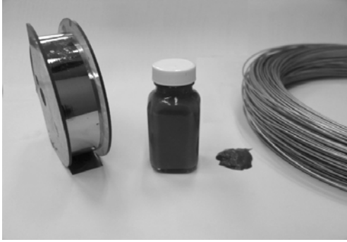
Fig. 1 Various brazing alloys (left: amorphous foil, middle: paste, right: wire)
