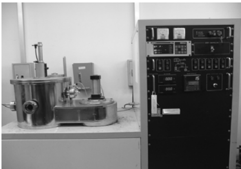
Fig. 6 Vacuum brazing furnace
