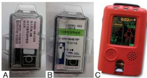
Fig. 1. A : Thermoluminescence dosimeter (TLD, Panasonic UD-802), B : Optically stimulated luminescence dosimeter (OSLD, InLight system, Landauer), C : Electronic personal dosimeter (EPD, Tracerco T404)
