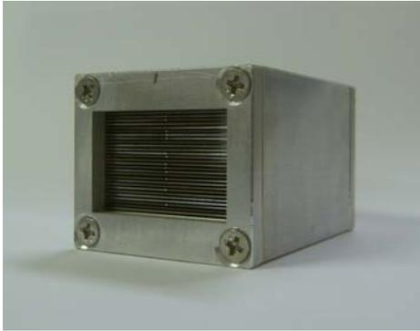
Fig. 5. Fabricated parallel beam optic for an X-ray diffractometer
