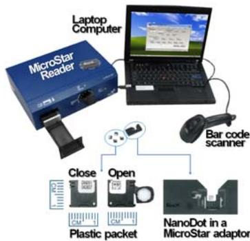
Figure 2. InLight™ OSL system. The MicroStar reader is a compact, lightweight, portable reader. OSLDs are plastic discs infused with crystals of Al<sub>2</sub>O<sub>3</sub>:C and little build-up in device itself.
