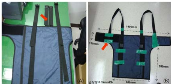
Fig1. Fabrication of lead apron for pregnant women (A) Attaching shoulder straps (B) New lead apron length
