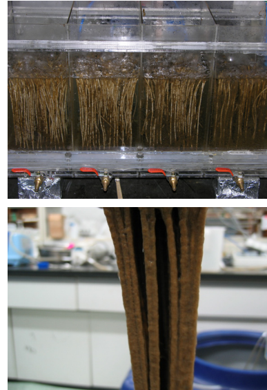
Fig. 12. Attached biofilm on the tube(Up : Initiation of biofilm formation, Down : Maximum of biofilm formation).
