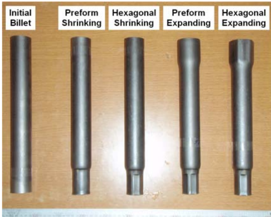
Fig.12 The intermediate and final forgings obtained by cold forging experiments
