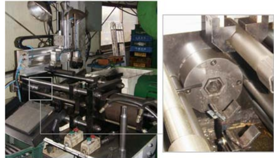
Fig.11 The manufactured forging machine based on the designed process sequece
