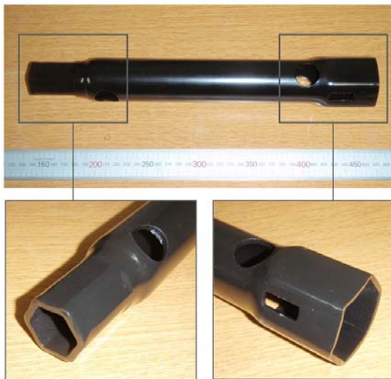
Fig.13 The final product of the hollow-type wheel nut wrench
