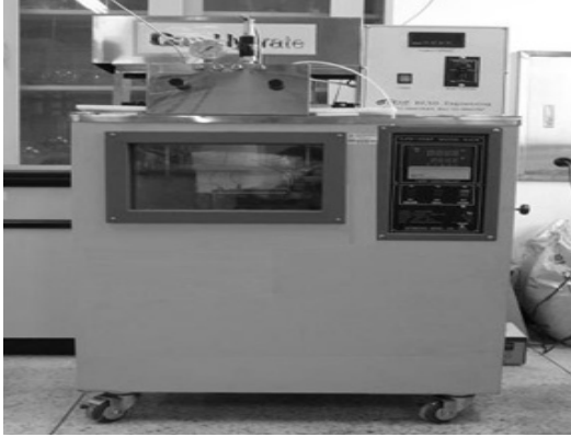
Fig. 3 Isothermal bath and gas hydrate reactor
