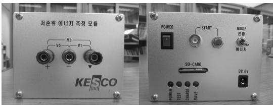
Fig. 6 The appearance of voltage absence and low level energy measurement device
