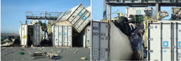
Fig. 3 Explosion of refer container
