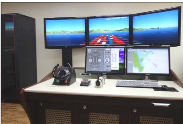
Fig. 6 LCD monitor, conning controller & operation server
