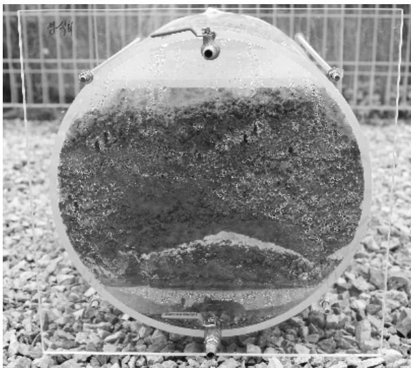
Fig. 3. Structure of modeled carcass burial site used in this study.
