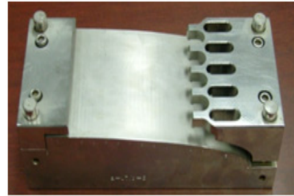
Figure 2. Photo of Bergen jig to give a strain in specimen.
