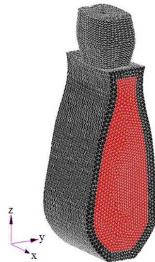
Fig. 7 Finite element model for dental implant analysis
