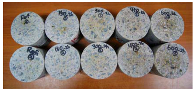
Fig. 4 Thermal damaged concrete specimens for nonlinear ultrasonic wave modulation
