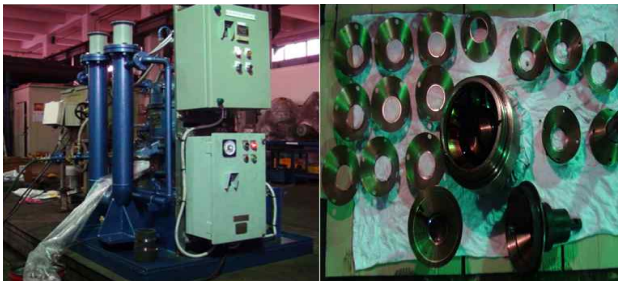
(b) Photo of sludge test bed and bowl with disc
