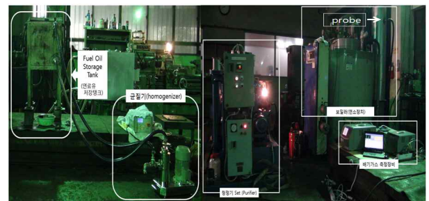
(b) Photo of exhaust gas measurement
