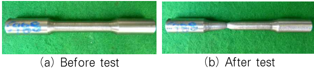
Fig. 1 Weld Metal Tensile Test Specimen
