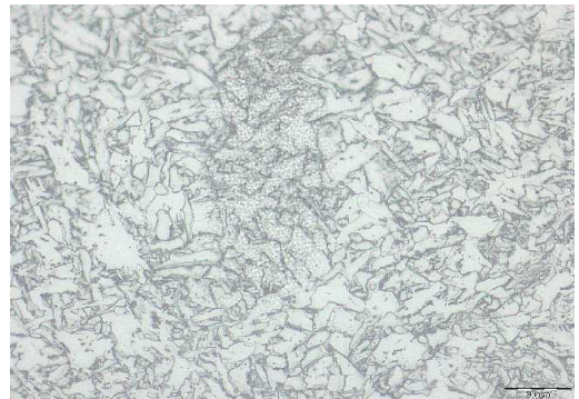
(c) Weld Metal(×500)
