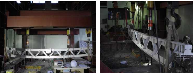
Fig. 7 ST600P Test Specimen at Maximum Load
