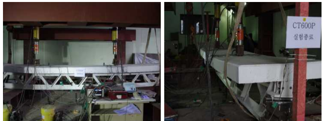
Fig. 11 CT600C Test Specimen at Maximum Load
