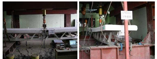
Fig. 9 CT600C Test Specimen at Maximum Load
