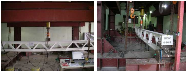
Fig. 5 ST600C Test Specimen at Maximum Load
