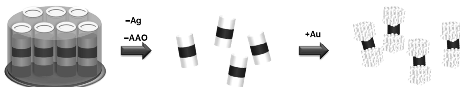
Scheme 1. The synthetic procedure of dumbbell-like Au-Ni-Au nanorods. Au-Ni-Au three-block nanorods were fabricated by the aid of anodic aluminum oxide template and electrochemical deposition. After releasing three-block nanorods, Au atoms were further selectively grown on Au surface of three-block nanorods by using solution-phase chemical growth.
