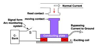
Fig. 1. The simplified mechanism of the Thomson coil type actuator.
