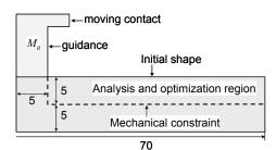
Fig. 4. Initial structure of plate and moving contact.
