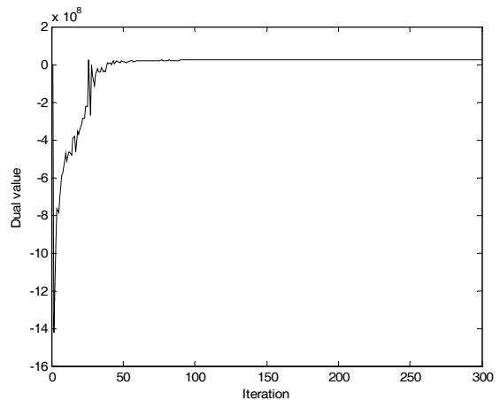
**Fig. 4.** Dual optimization convergence locus based on CP for case UK100\_24 – overall view
