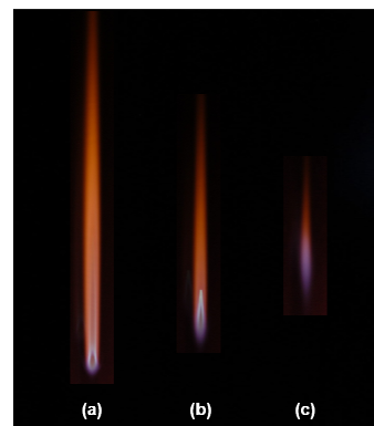
Fig. 1 Direct photographs of autoignited lifted flames at (T_0, R_H, U_0) = (980 \text{ K}, 0.02, 20.0 \text{ m/s}) for X_{F,0} = 0.20 (a), 0.15 (b), and 0.10 (c)
