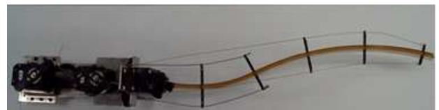
Fig. 1 Fish robot tail made by Urethane
