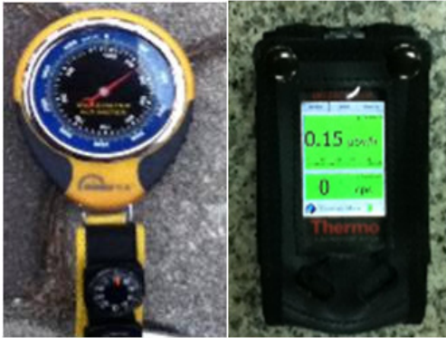
Fig. 2 The measuring instrument of gamma dose: INTERCEPTOR TM (Thermo, USA, 2006) (left), An altimeter: MINGLE (China, 2011) (right).
