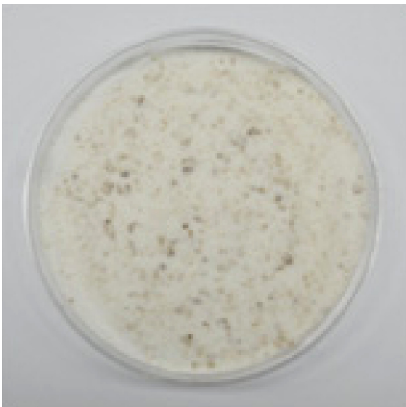
Fig. 2. Dry yeast manufactured by Spray Dryer(Y111-5).
