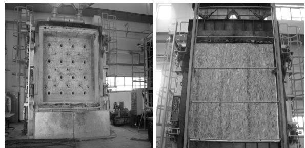
Fig. 7 A view of the furnace and specimen
