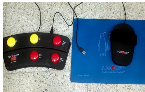
Figure 4. A foot mouse used in this experiment
