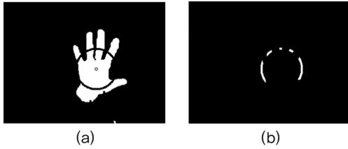
[Fig. 3] Finger detection using center point of palm and the circle
