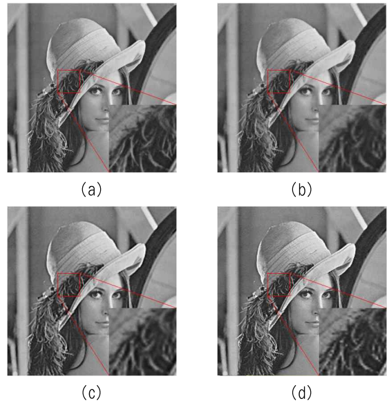
Fig. 5. Subjective quality comparison on enlarged "Lena" image (a) Original (b) Bicubic (c) Back projection (d) Proposed
