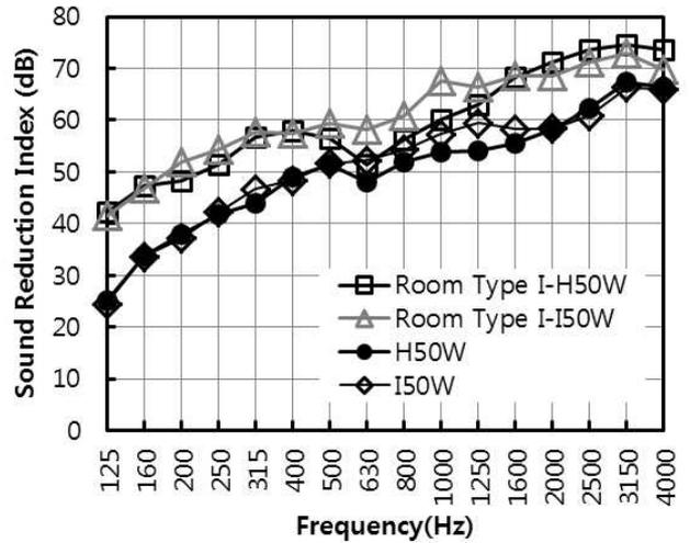
Figure 10. Comparison of sound reduction index between room type I and room type II
