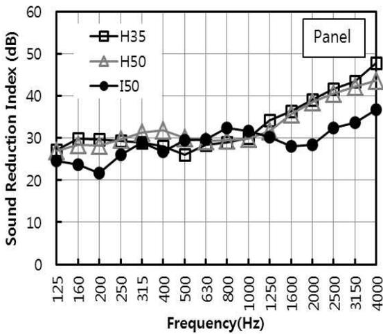
Figure 8. Sound reduction index according to section shape of extruded panel
