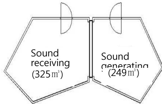
Figure 1. Floor plan of the reverberation chamber of room type I
