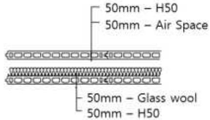
(b) Sectional view of H50W wall module
