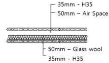
(a) Sectional view of H35W wall module
