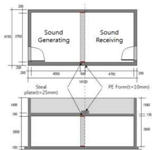
Figure 3. Design condition of room type II
