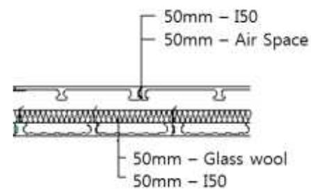
(c) Sectional view of I50W wall module
