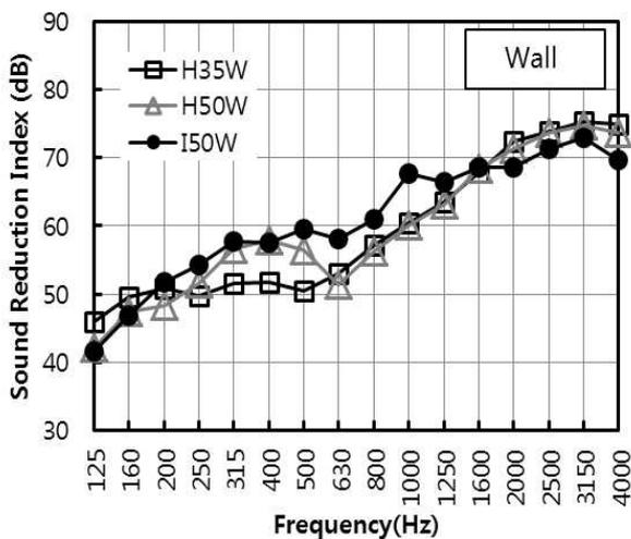
Figure 9. Sound reduction index according to wall type
