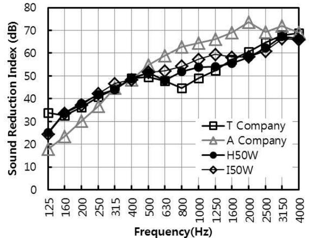
Figure 11. Comparison of sound reduction index between commercial products and this study
