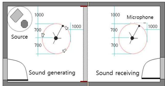
Figure 2. Floor plan of the reverberation chamber of room type II
