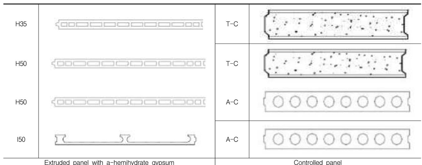
Figure 4. Section of panel used in sound insulation test
