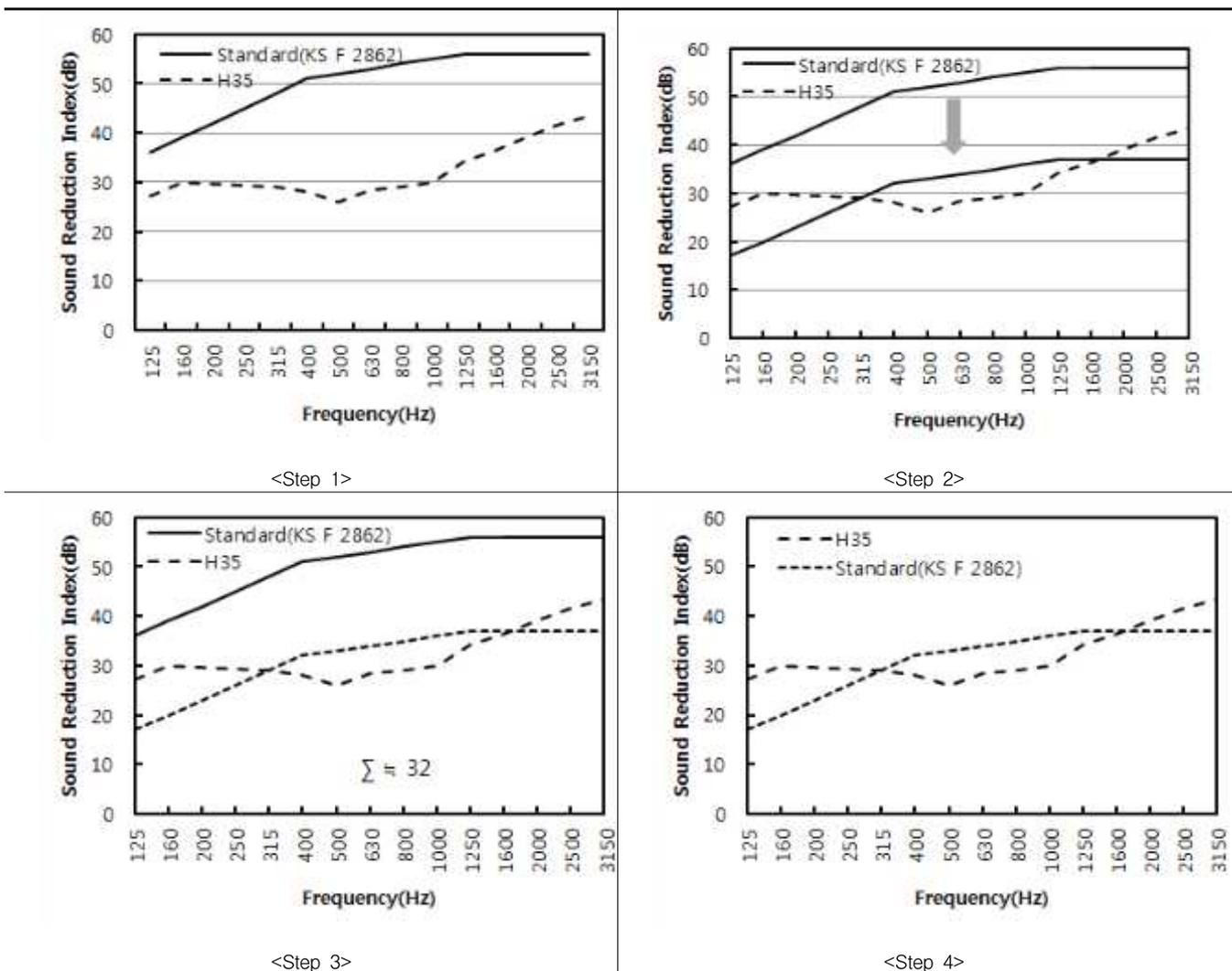
Figure 7. Calculation methods of single-number quantity for airborne sound(Ex. H35)
