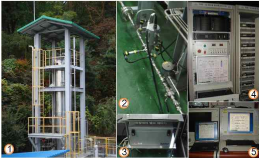
Fig. 18. Thrust control simulator (1:run tank, 2:TCV, 3:TCV controller, 4:DAS, 5:console)
