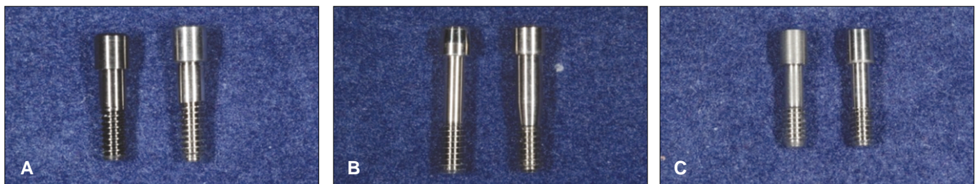
Fig. 2. Representative of the control and experimental group. For the Prefabricated (left) and customized (right) Titanium screws (A, B, C).
