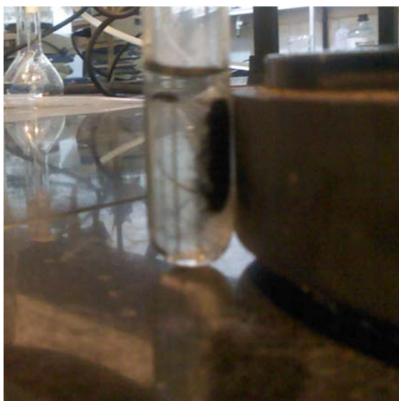
Figure 1. Immediate response of prepared magnetite nanoparticles to the permanent magnet.
