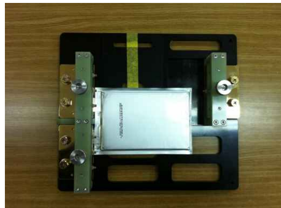
Fig. 7 Li-PB Battery 6.5Ah cell for HEV
