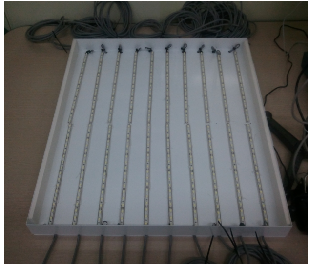
FIG. 1. Photograph of the white LED lighting composed of 360 PC white LEDs where 18 LEDs were grouped as a channel, and hence, the number of channels was 20 in total.
