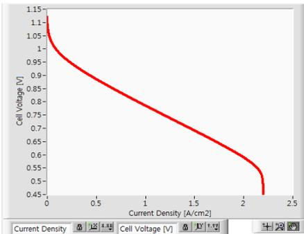
Figure 3: Polarization Curve Simulation.
