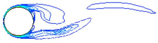
Figure 8(a): Vorticity contour moving cylinder at Re=50 and a=2.0
