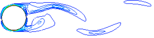
Figure 9(b): Vorticity contour moving cylinder at Re=100 and a=1.0
