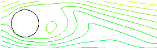
Figure 7(a): Streamlines of flow over fixed cylinder at Re=100
