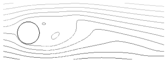
Figure 6(a): Streamlines of flow over fixed cylinder at Re=50
