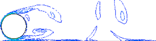
Figure 9(c): Vorticity contour moving cylinder at Re=100 and a=0.6
