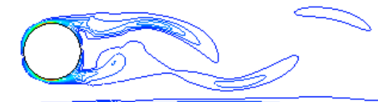
Figure 8(b): Vorticity contour moving cylinder at Re=50 and a=1.0
