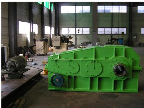
Figure 5: Decelerator for Briquetting Machine.
