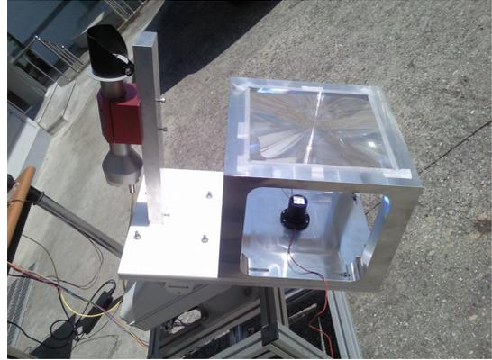
Figure 2: Fresnel lens performance test
